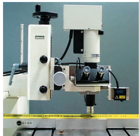
Fig. 3: Electro-optical micro-scope for edge detection
