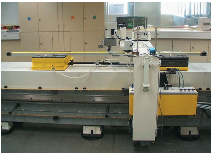
Fig. 2: The horizontal comparator for staff calibration at UniBwM
